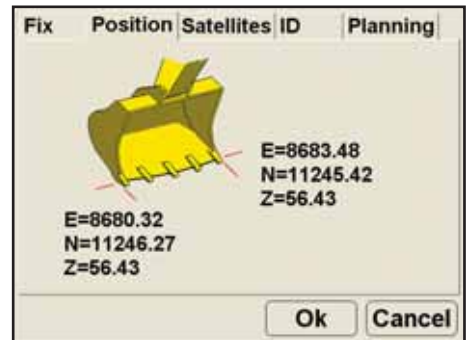
See the coordinates of both sides of the bucket's cutting edge
